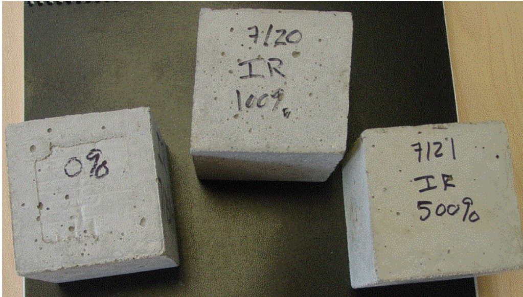
Figure 3. Concrete cubes with known chloride concentrations, prepared at Rutgers, Cubes are 3" on a side.
