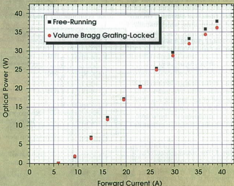
Figure 4. The total output power of a free-running laser diode bar and the off-the-shelf 40-W locked LuxMaster laser diode bar are compared.
